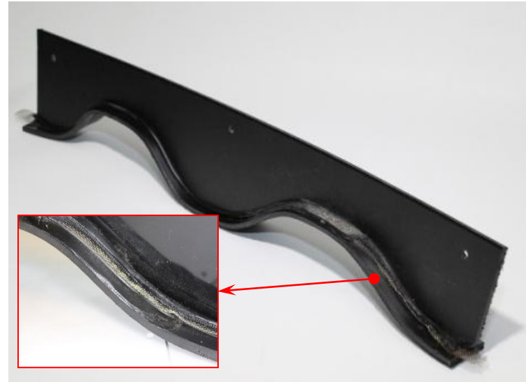
Specimen of a T-welded joint with complex geometrical surface
